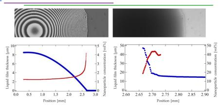
We succeeded in simultaneously measurement of liquid film shape with a thickness of nm to  $\mu m$  and the areal distribution of nanoparticle concentration.
