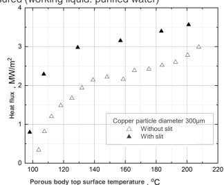
For boiling on a plane heated surface in water at atmospheric pressure, the critical heat flux is  $1\,\mathrm{MW/m^2}$
