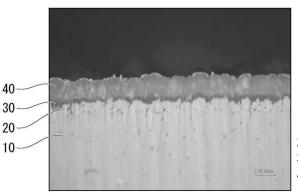
10.Substrate (SiC)20.CVD-SiC layer30.Buffer layer40.Coating layer (alumina)
