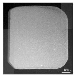
Even after the corrosion test, the coating did not peel off and no trace of corrosion was observed.
