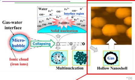
The nanoshells with fine uneven surface were observed by AFM.
