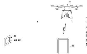
10. Moving object 11. Imaging unit 20. information processing device MK Marker MK1 1<sup>st</sup> marker MK2 2<sup>nd</sup> marker
