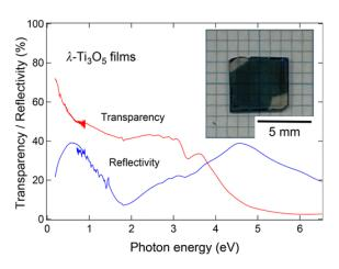
Optical spectra of the  $\lambda$ -Ti<sub>3</sub>O<sub>5</sub> films. The inset shows the photograph of the films. The films are not deposited at the top-left and bottom right sides because the cramps cover the surface of the substrates during film deposition.
