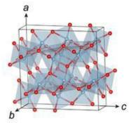
Schematic crystal structure of  $\lambda$ -Ti<sub>3</sub>O<sub>5</sub> drawn by VESTA
