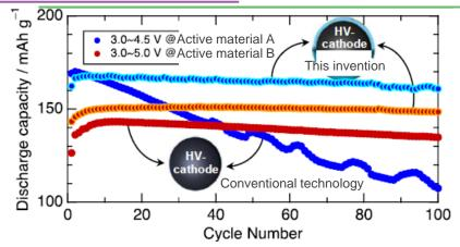
Able to obtain charge/discharge cycle characteristic without degradation for more than 100 cycles by coating the surface of the cobalt-free spinel oxide active material for 4.7 V class cathode with a fluoride solid electrolyte layer.
