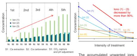
Recycling use of the extraction solution leads to accumulation of unwanted ions
