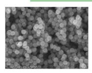
It is possible to produce spherical zinc oxide in which particles with a primary particle diameter of 2~200 nm accumulate to form spheres of 20~5000 nm.
