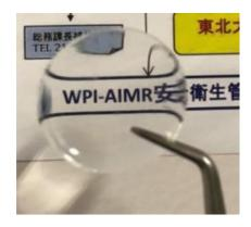
\*This electrolyte shows 10% elongation at very low force, with a maximum elongation of 30%. It also shows high ionic conductivity of  $2.7x10^{-5}$ S/cm at room temperature and  $2.1x10^{-4}$  S/cm at 60°C.
