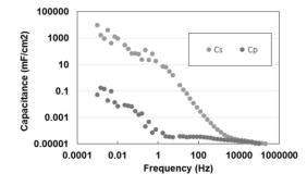
[Up left]Diagram showing the molecular structure of ultracapacitor material and the electric distribution constant circuit [Up right]X-ray diffraction patterns on the surface of ultracapacitor material [Down left] Frequency response of storage capacitance Cs in a series junction and Cp in a parallel junction for ultracapacitor material
