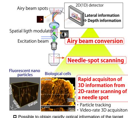
Possible to obtain rapidly optical information of the target sample from different positions along the optical axis
