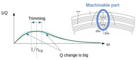
Adjust the Q factor by machining the machinable part
