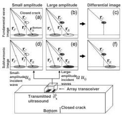
In (c), only the crack ( $\mathbf{r}_{\rm C}$ ) can be visualized by utilizing the nonlinear characteristics of fundamental wave, while the ghost ( $\mathbf{r}_{\rm R}$  in (f)) in the subharmonic image is removed.
