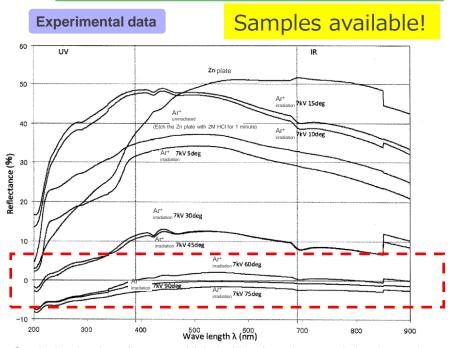
Graph showing the reflectance of light incident from the normal direction on the zinc plate treated under each condition
