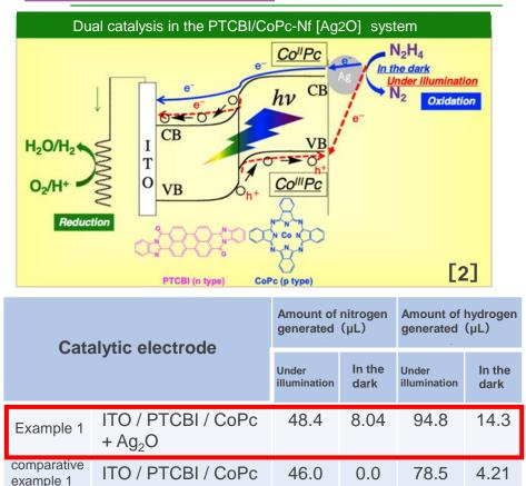
Both under illumination and in the dark, hydrogen generation associated with the oxidation of hydrazine can be confirmed, and it is larger under illumination than in the dark.
